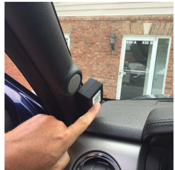
6. Unit mounted on A-pillar using provided 3M tape with OBD extension cable tucked behind dashboard
