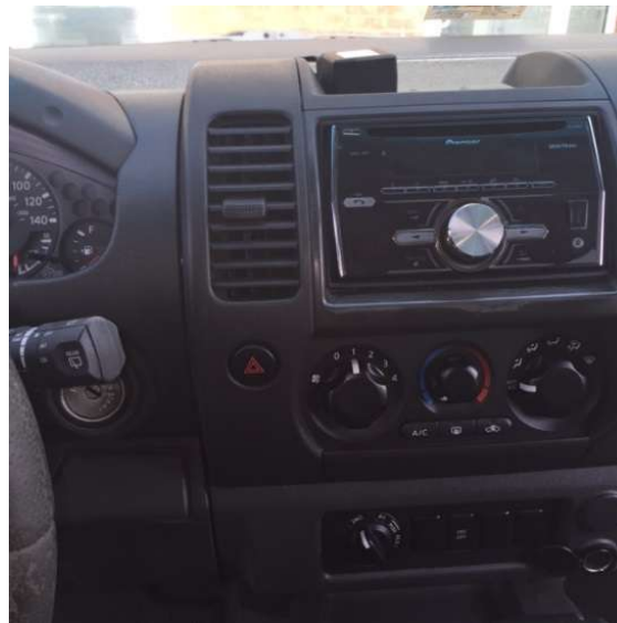
5. Unit mounted above radio with OBD extension cable tucked behind dashboard
