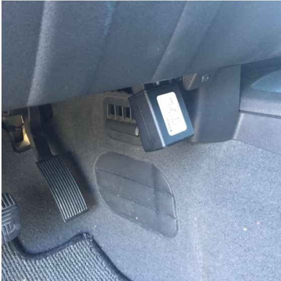
1. ODB installation without strap
