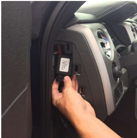
4. Unit with OBD extension cable tucked completely behind the dashboard
