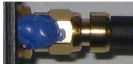
Anti-Sabotage Lacquer applied to connector.
