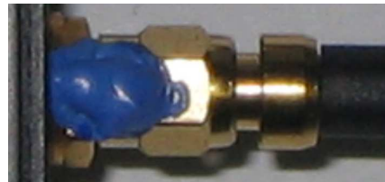
Anti-Sabotage Lacquer applied to connector.
